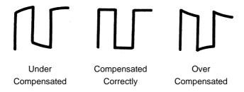
Use a nonmetallic flat-head screwdriver to adjust the low-frequency compensation adjustment hole on the probe until the waveform matches the "Compensated Correctly" waveform above.
