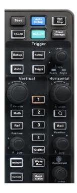
The front panel is designed to operate the basic functions without having to open the software menu. Most of the front panel controls duplicate functionality available through the touch screen display but the operation is more quickly achieved
